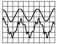
This is a variety of harmonic frequencies superimposed on the desirable sine wave frequency passed back along the local power grid to other equipment throughout an entire office building or local neighborhood. The effect is measured by % VTHD, a measure of the amount of voltage variation within the waveform.
